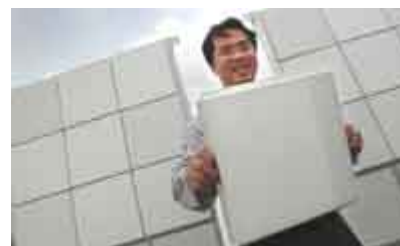
This aluminium plate Dr Chris Cai holds has been exposed to the elements for six months and the portion with the self-cleaning coating appears whiter. -- JOYCE FANG
